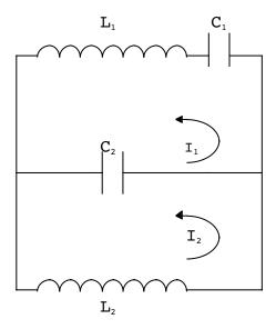
If we rewrite Eqs.(3.62) in terms of the spring diplacement variables instead of mass diplacement variables, we would have found the same circuit but with individual currents running across the capacitors rather than the inductors.
