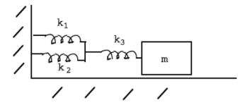
Using the circuit/mechanical analogy, find the equivalent circuit to this mechanical oscillator.
